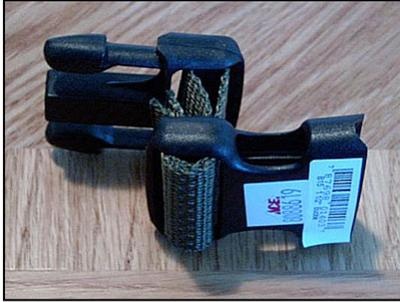
4. Assemble this piece using the 5 or 7" piece of 1.5" wide web and the female and male ends of 1.5" buckles. Pay close attention to the web's routing and the direction of the buckles. If desired, cut down the webbing after the threading process.
